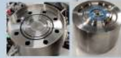
The high-pressure cell with insert for foil measurements (left) and insert for O-Ring measurements (right)
