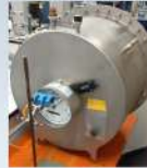
The reference systems for gas meter calibration: pVT-t system, CESAME, France (left); drum-type gas meter VSL, Netherlands (right)
