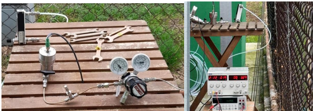
Figure 19: NPL oxygen sensor setup at Turin Airport.
