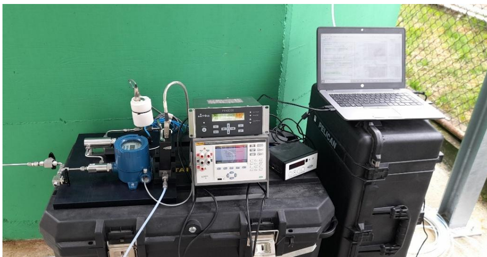
Figure 16: INRIM humidity sensor setup at Turin Airport.
