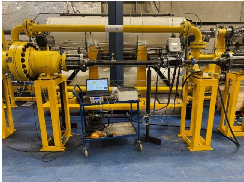
Figure 6. Testing of the ultrasonic meter at FORCE
