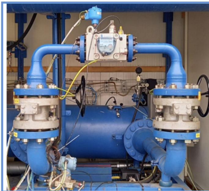
Figure 4. Test facility at VSL with the rotary meter at the meter-under-test position, with a part of the prover tube in the background
