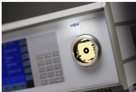
Figure 4: A photo of an MBW 373 chilled mirror hygrometer (source Process Insights).
