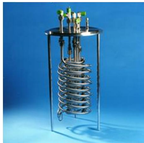
Figure 1: NPL Multi-gas, Multi-pressure Primary Standard Humidity Generator
